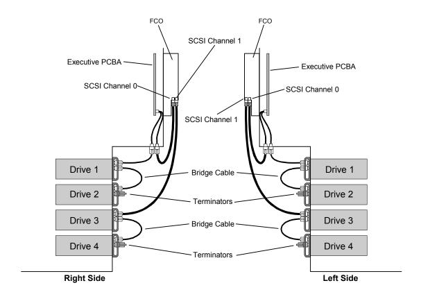
Figure 6-8 TLS-58xxx, 68xxx and 88xxx Cabling Diagram
